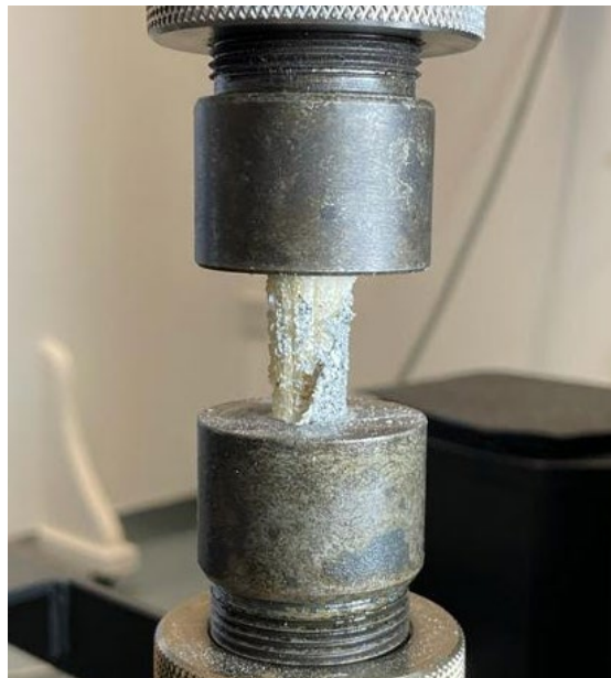
Figure 2: GFRP bar subjected to compressive loading.
