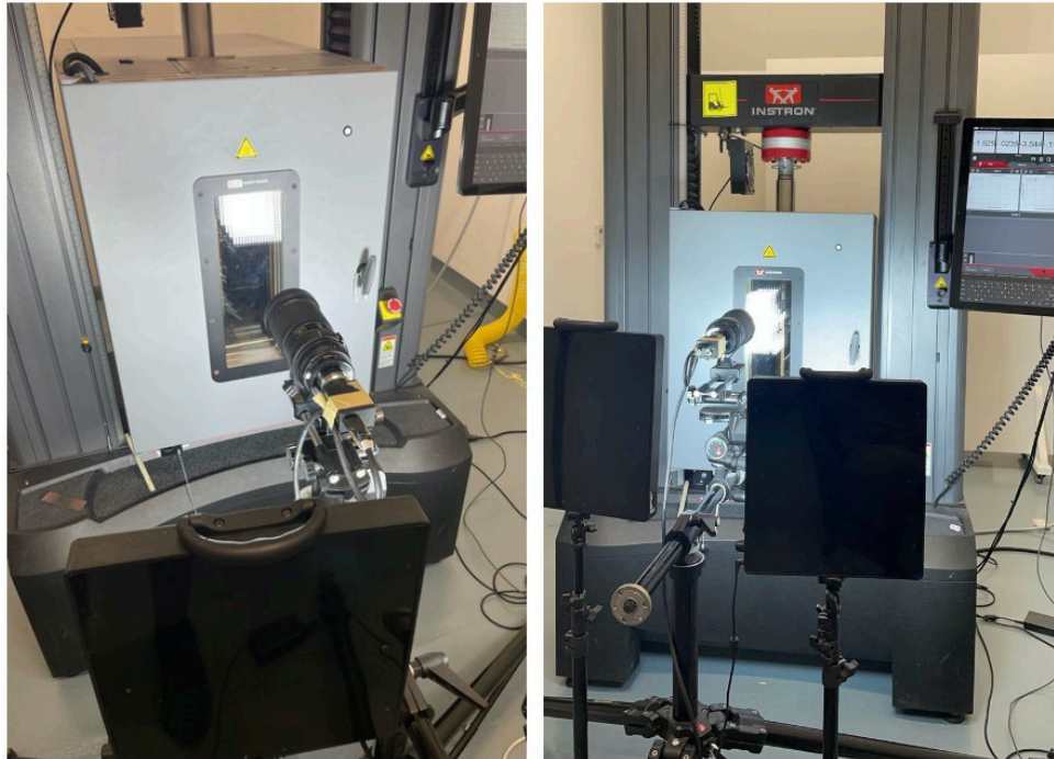
Figure 1: Test set-up using the DIC machine.
