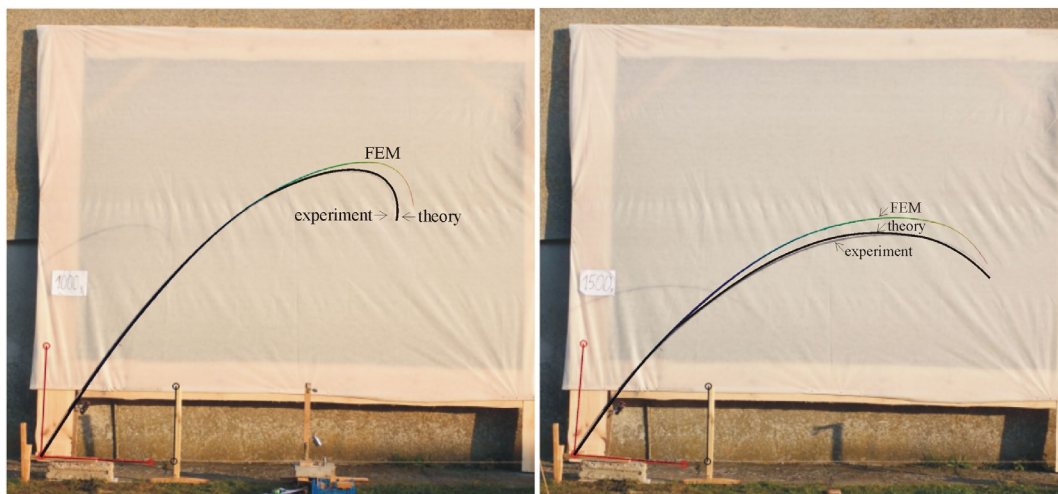
Fig. 6. Comparison of experimental, FEM and theoretical results for two selected combinations of load magnitudes and distances
