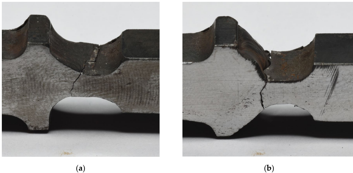
Fig. 7. Selected stages of crack development in a weld specimen with HT: (a) concave welds, b) convex welds
