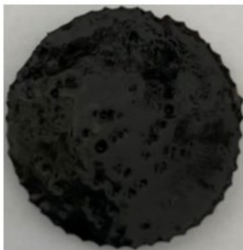
Figure 6. A cured product using resin degradation products of Entry 7 and unsaturated polyester.
