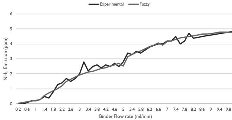
Fig. 5: Graph of comparison value of the NH<sub>3</sub> Emission
