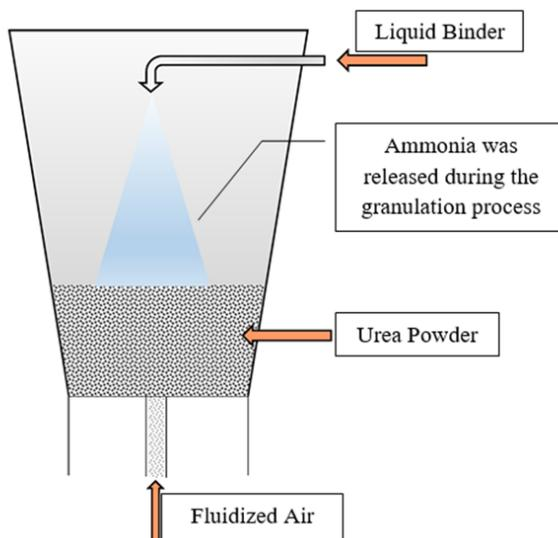
Fig. 1: Schematic of fluidized bed granulation process
