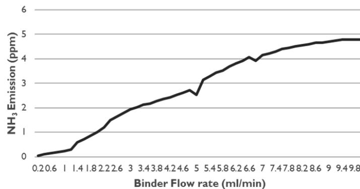
Fig. 4: Graph on NH<sub>3</sub> Emission vs Binder flow rate
