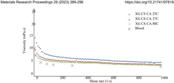
Fig. 2. Viscosity against shear rate for xanthan gum-corn starch-water glycerol base and contrast agent with variation of mixing temperature.
