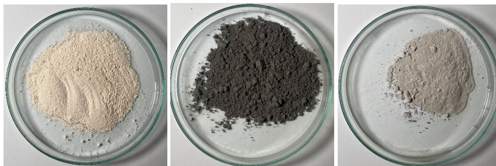
Fig. 3. Chicken eggshell powder before calcination (a), and after calcination at (b) 700°C and (c) 900°C
