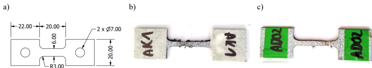
Fig. 1. The sample dimensions used in tensile tests (a) and samples after quasi-static (b) and dynamic (c) tensile tests.
