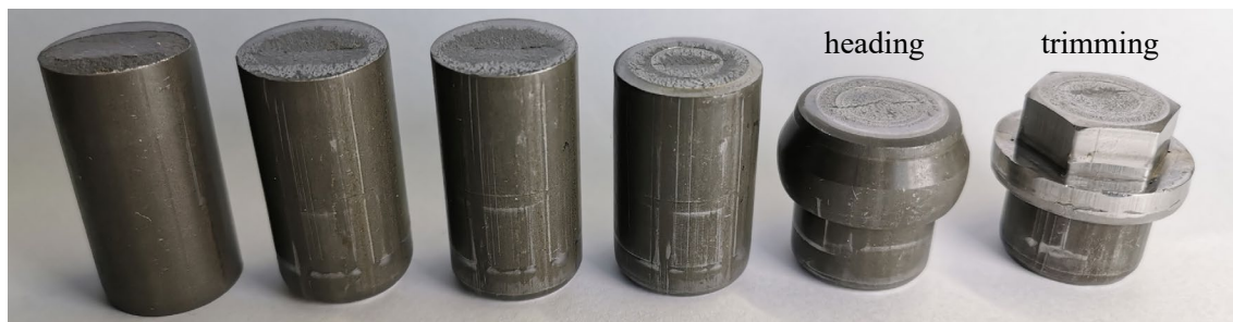
Fig. 6. Multi-stage process for production of a hexagonal screw with flange.
