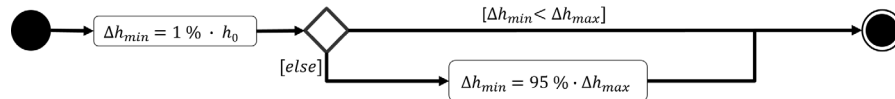
Fig. 5. Calculation of minimum height reduction \Delta h_{min} to guarantee reaching the desired final height.
