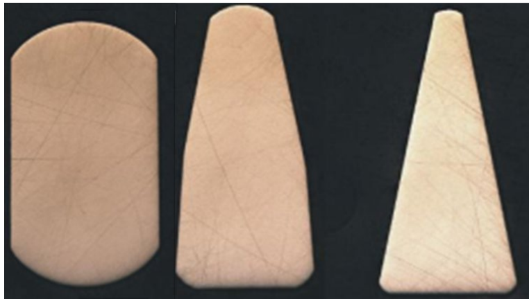
Fig. 4. Shape analysis of the rolled profile wires after each step of deformation.
