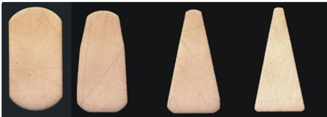
Fig. 2. Analysis of the shape of drawn profile wires after each stage of deformation.
