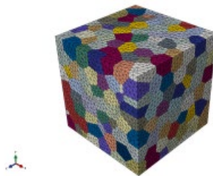
Fig. 2. 500 grained calibration cube model for homogenization.
