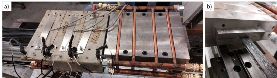
Fig. 3. a) Pultrusion setup while processing glass-polypropylene tapes; b) obtained pultruded profile.
