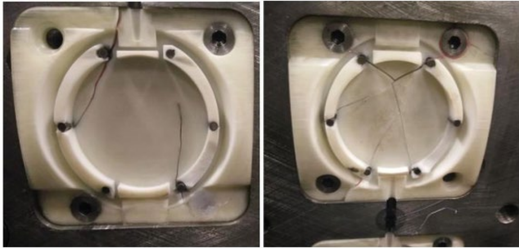
Fig. 11. MJF mold inserts with cracks after 40 molding cycles using HDPE and other 6 successful molding cycles using ABS as the molding material.
