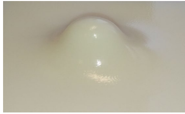
Fig. 1. Photopolymer model utilized to get the digital information by 3D SCANNING.
