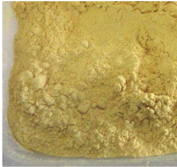
Fig. 2. CFREP powders as a feedstock for consolidation via the cold, dry stamping to a green compact.
