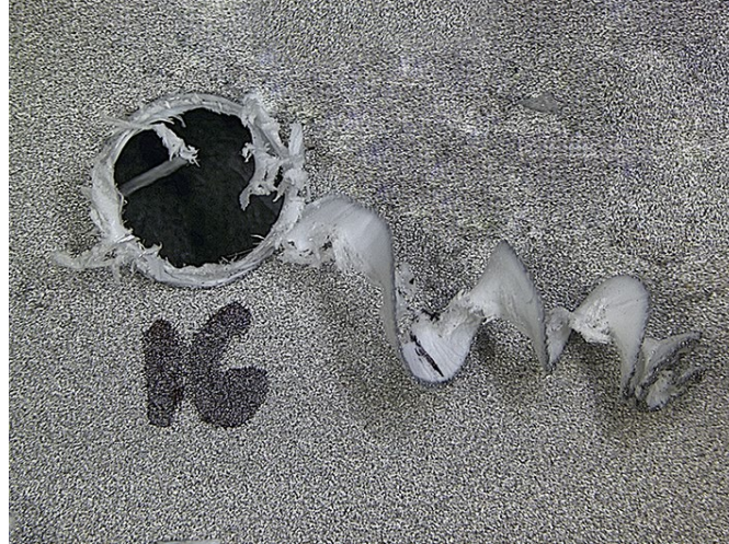
Fig. 4. Long continuous chip obtained with high values of the feed rate.
