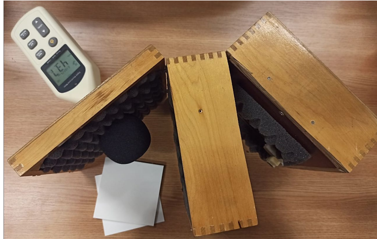
Fig. 3. Image of equipment used to study the influence exerted by some factors on the transmission of sound through small panels manufactured by 3D printing.
