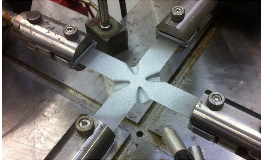
Fig. 4. Experimental setup with the pre-deformed cruciform sample.
