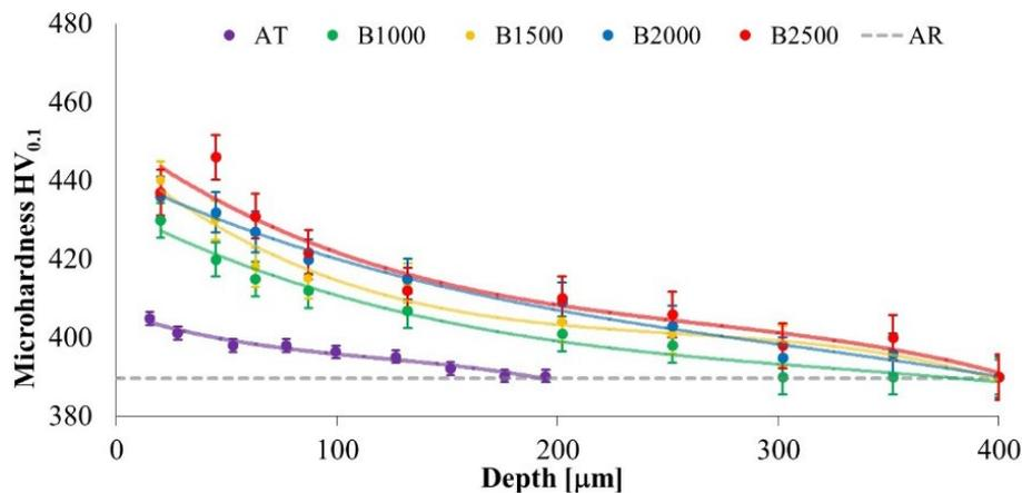
Fig. 5. Microhardness below the machined surface at varying burnishing force.
