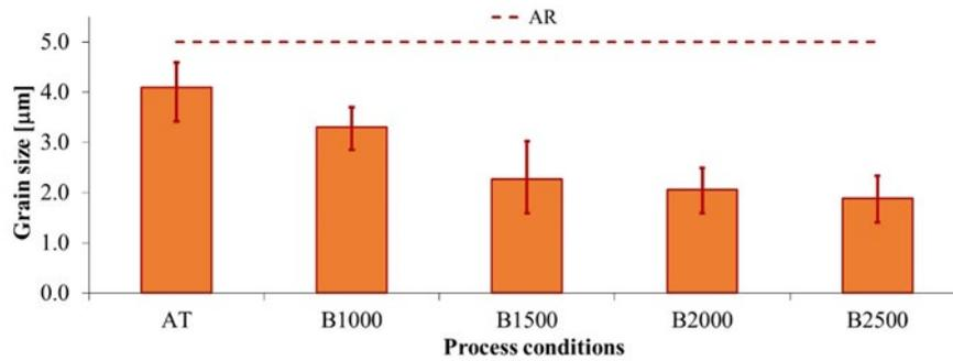
Fig. 3. Grain size evolution at varying burnishing force.
