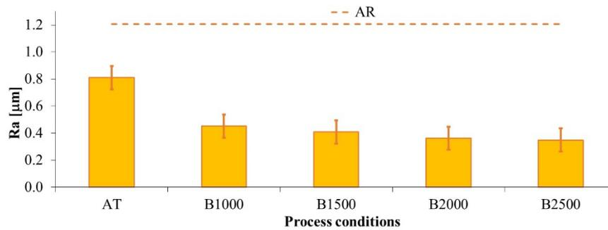
Fig. 4. Roughness at varying burnishing force.
