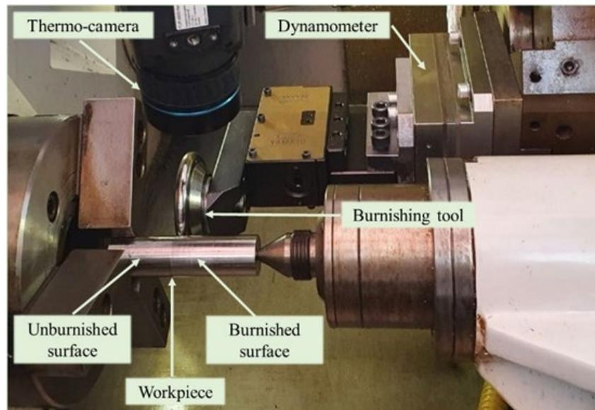
*Fig. 1. Burnishing process set-up.*
