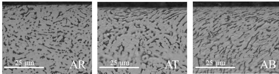
Fig. 2. Microstructure of the AR, AT and AB samples.
