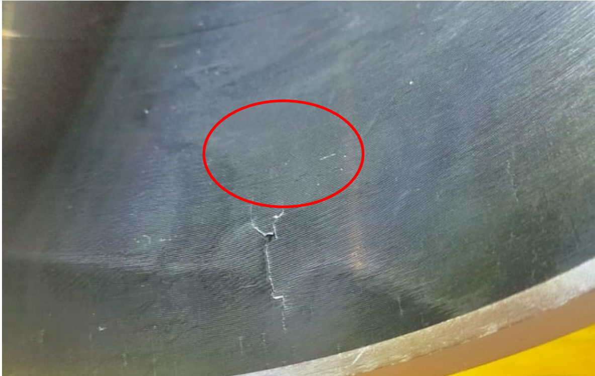
Fig. 4. Small surface crack formed inside QT sample.
