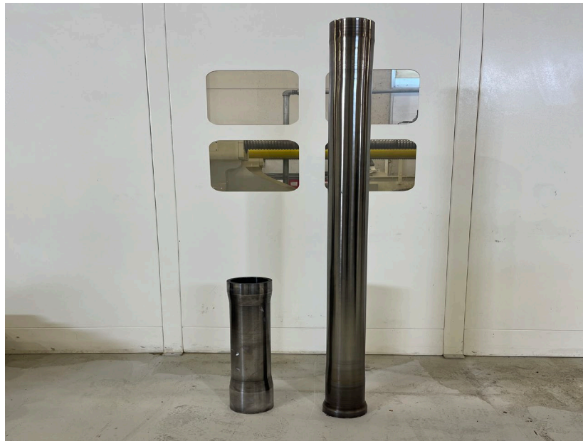
Fig. 1. Preform tube (Left) and flow formed tube (Right).
