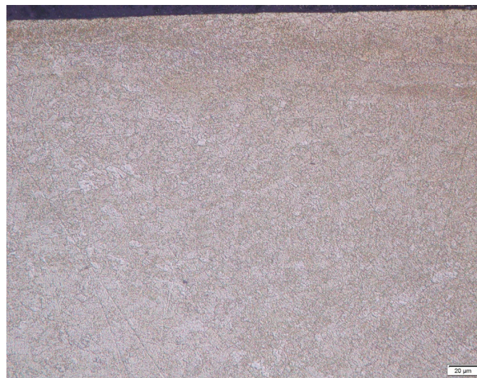
Fig. 6. FF1 heat treated at 350°C taken at 500X, Acidic Ferric Chloride-1min.
