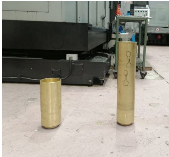
Fig. 1 Preform (PRE) part on the left and Flow-formed (FF1) on the right.
