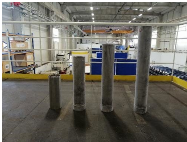
Fig. 1. General view of the preform (left) and flow formed 6082 Al tubes with increasing reduction ratios of 45%, 55%, and 65% from left to right.
