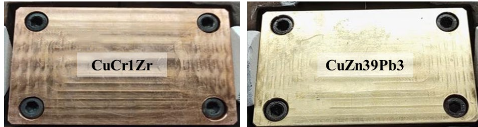
Fig. 2. Contact plates made of different materials.
