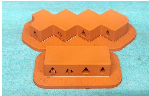
Fig. 4. Green state of the manufactured straight and angled test parts.
