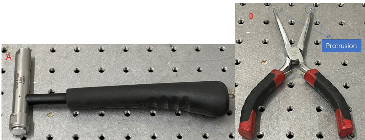
Fig.6 Instrument used in the experiment: (A) Impact hammer. (B) Custom-made plier
