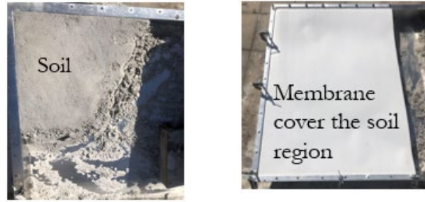
Figure 4: Test fixture showing installation of simulated scum-berg and membrane over simulated scum-berg
