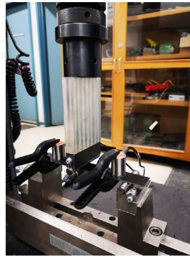
Figure 2: Experimentation setup for three-point bend test on composite specimens.
