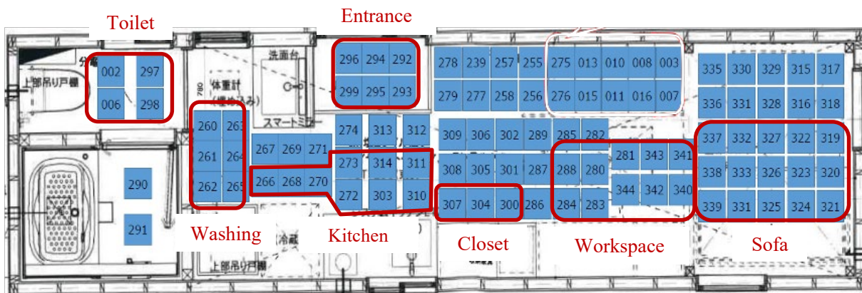
Figure 2. The locations of the ground reaction force sensors and defined seven zoning areas
