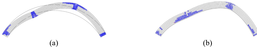
Figure 7 Crack pattern at the failure load of the unreinforced arch ( T_z=0.6 mm) (a) Unstrengthened arch and (b) strengthened arch
