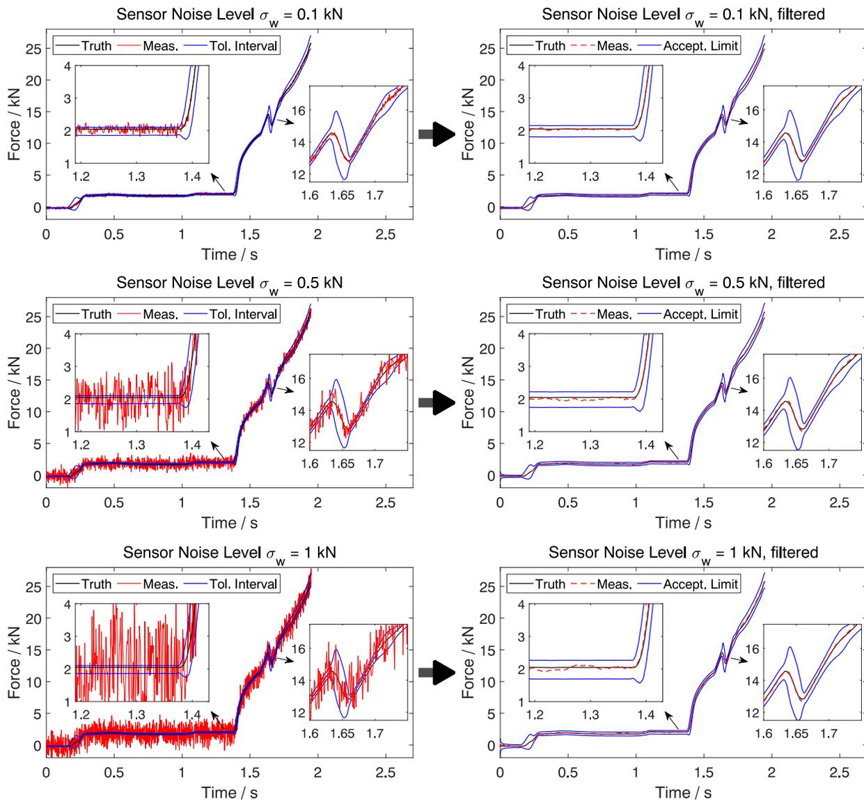
*Fig. 3: Results for the material combination St-Al. Left: Simulated process curves with different noise level (red curve) and indicated tolerance interval (blue curves). Right: Filtered signal (extended Kalman filter, red curve) and indicated acceptance limits (Tolerance interval extended with guard bands that depend on the uncertainty output from the Kalman filter, blue curve) for a probability of non-conformance of 95 %.*
