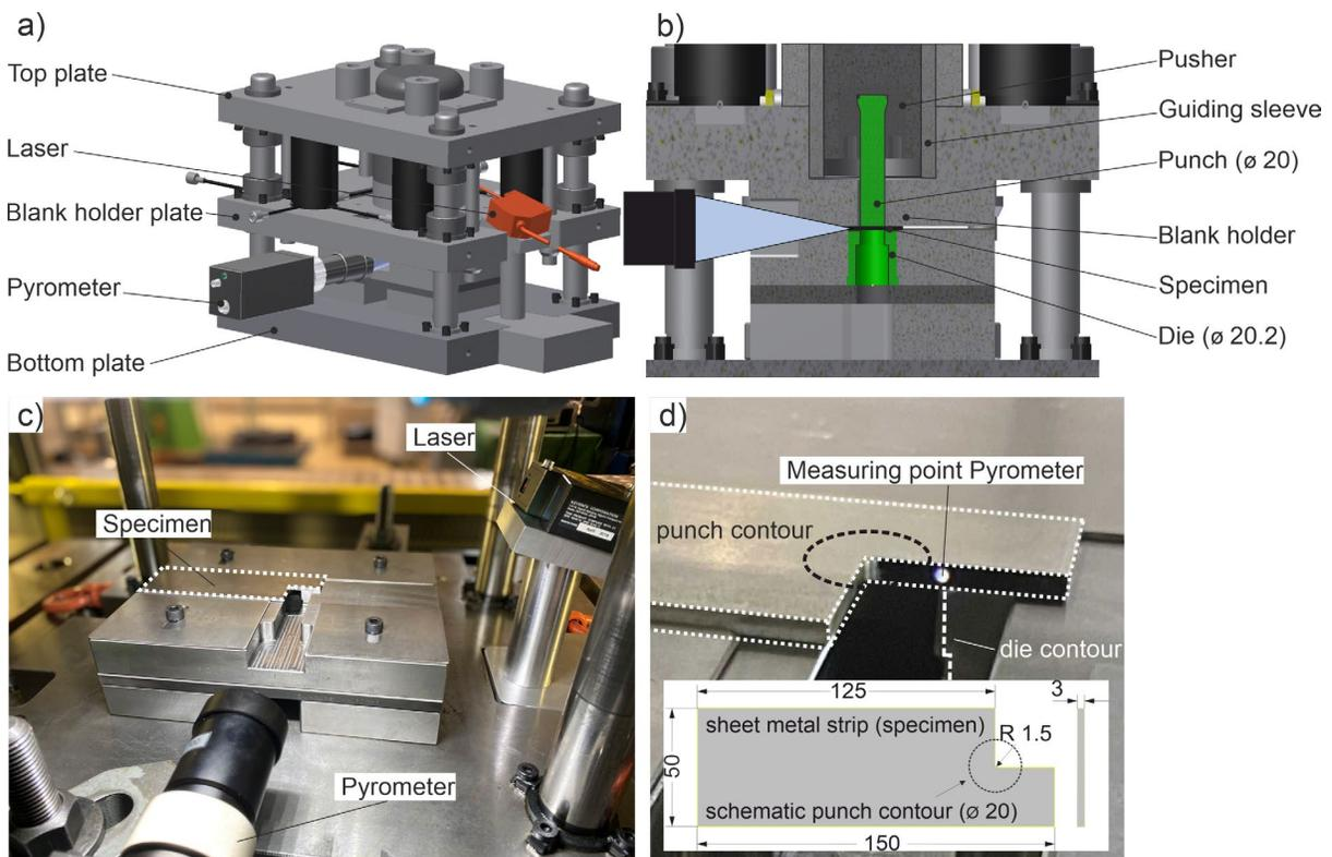
*Fig. 1: Experimental setup for the HSIC tests. a) and b) CAD drawing of the tool with positioning of the measuring equipment and the relevant components. c) and d) Specimen geometry and position of the measuring point of the pyrometer.*
