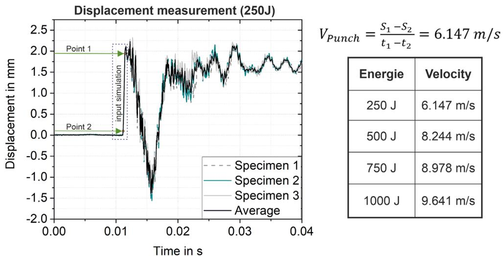
Fig. 3: Representative displacement-time measurements at an energy level of 250 J. The gradient of the curve between point 1 and 2 corresponds to the velocity and were used as input parameter for the numerical simulation. The measured velocities from 250 J to 1000 J are recorded in the table.
