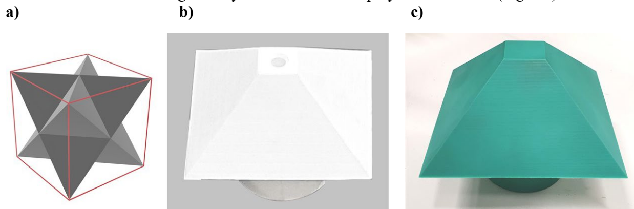
Figure 1: a) unit cell of the octet infill pattern b) 3D printed die c) milled die
