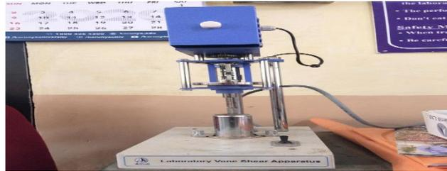
Fig 3 Vane shear apparatus
