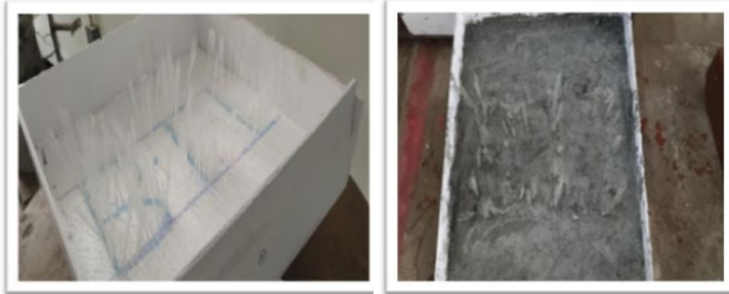
Figure.6 Placing of Optical Fiber in Concrete.
