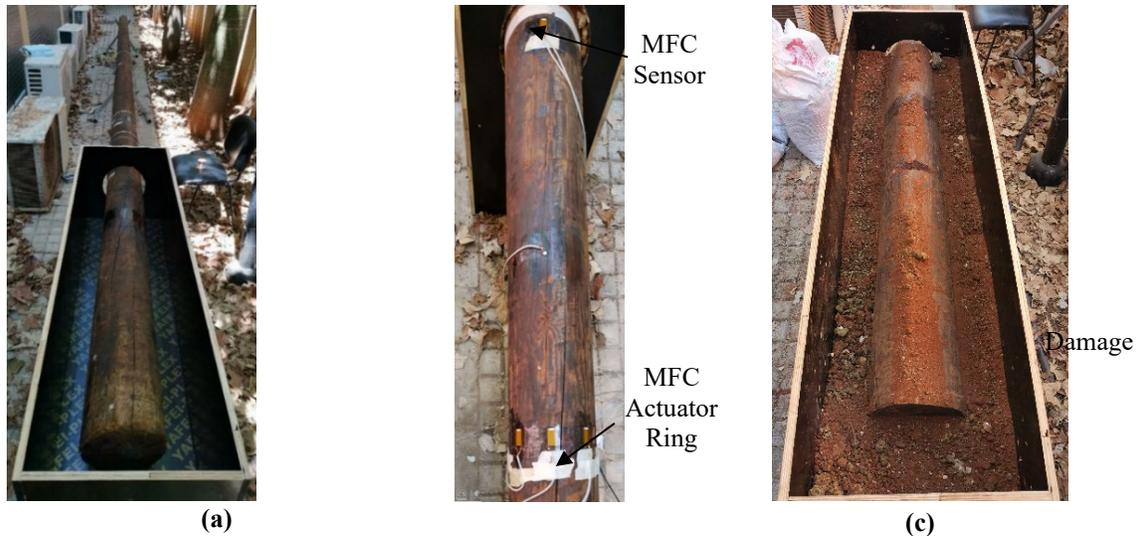
Fig. 3 (a) 8-meter timber utility pole, (b) MFC actuator ring and sensor configuration and (c) Induced damage in the embedded section of the pole.
