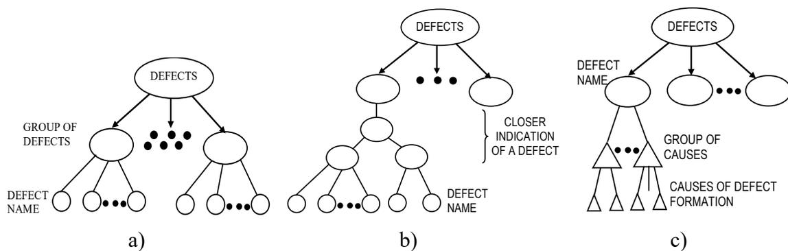
Figure 1. Classification diagrams for casting defects in classic materials [17-21]
