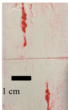
Figure 1. Reference image of cracks in Block 6 revealed by dye penetrant testing.
