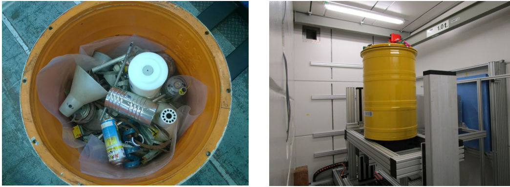
Fig. 1: Left: Open 200-l drum during assembling with two pellets covered by scrap. The white PE-cylinder can ingest neutron sources. Right: 280-l drum on the sample manipulator of NECTAR.
