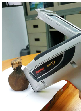
Fig. 3 The elemental analysis by using a handheld XRF spectrometer.
