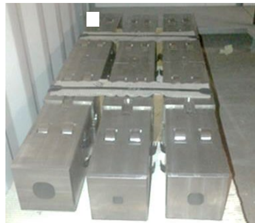
Fig. 2. Three B-Fe collimators: with different aperture openings ( D ) of 12 mm, 24 mm and 42 mm respectively.
