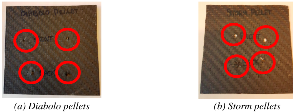
Figure 8-Visual inspection of the impact
