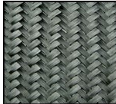
Figure 2-Carbon fiber twill weave
