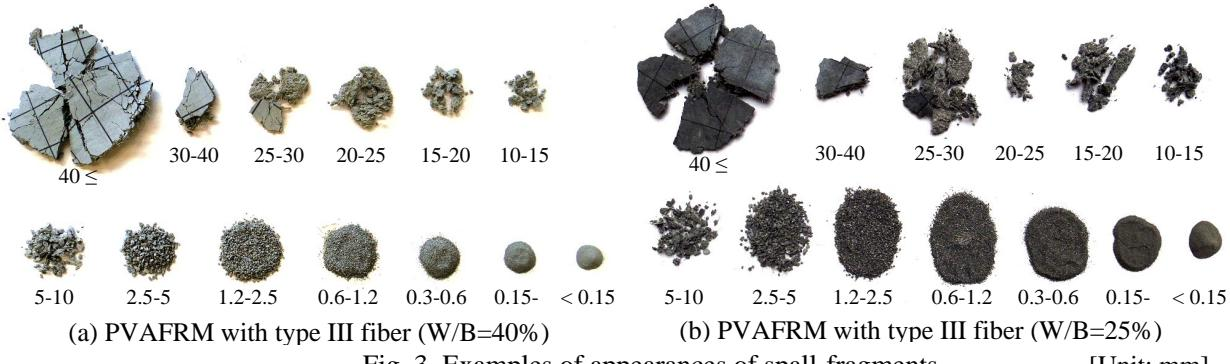
(a) PVAFRM with type III fiber (W/B=40%) (b) PVAFRM with type III fiber (W/B=25%)
