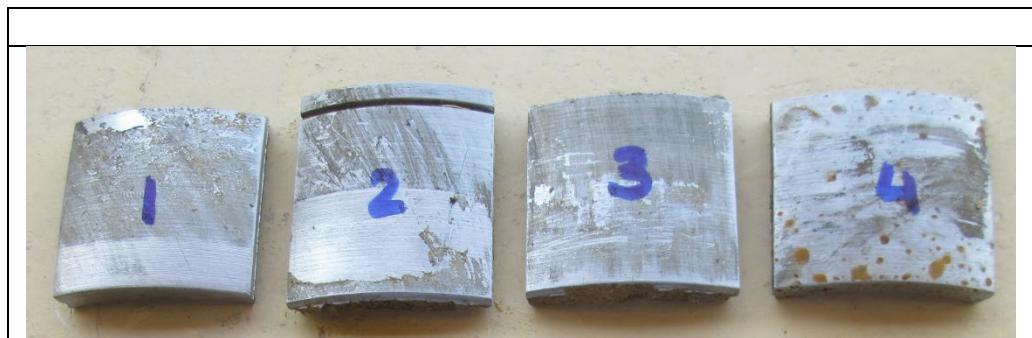
Figure 4. 3-kg class Prototype Warhead and Fragments
