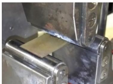
Fig.8 Three-point bending test
