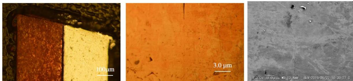
(a) Corrosion of Cu and Al. (b) Optical of corroded Cu. (c) SEM of corroded Cu.
