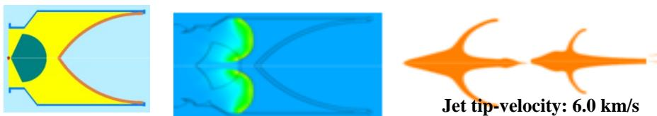
Fig. 8 Formation of Jet-tip velocity from Tulip shaped charge warhead
