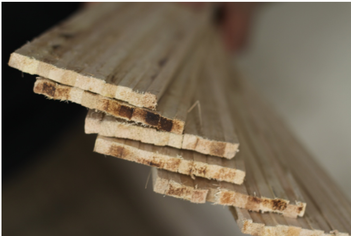
Fig. 23: Boards from palm midribs.
