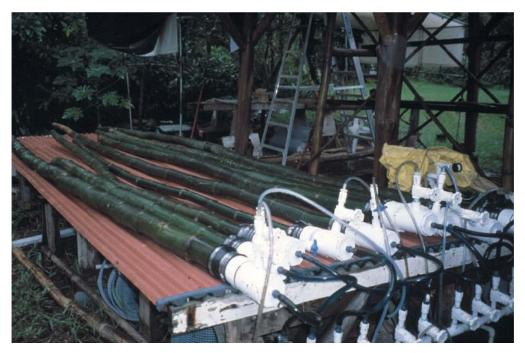
Fig. 7 The sap-replacement method requires an air suction/pressure cap at the culm end.
