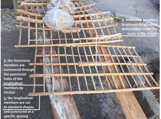
Figure 1 Bread crates made from Date Palm Midribs.
