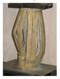
Fig. 2 Culm internode crushed under load.
