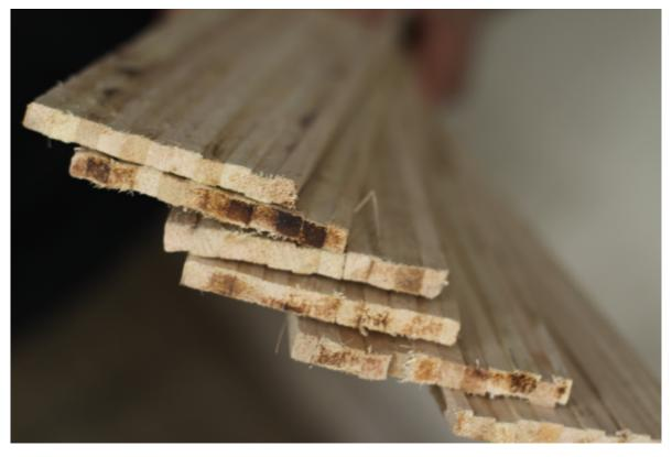
Fig. 23: Boards from palm midribs.
