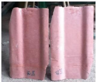
Fig. 1. Samples of coconut husk fibre-reinforced roofing tiles.
