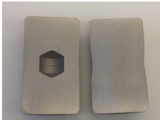
Fig. 3. Cross section of artificial pore before HIPing (left) and after HIPing (right).
