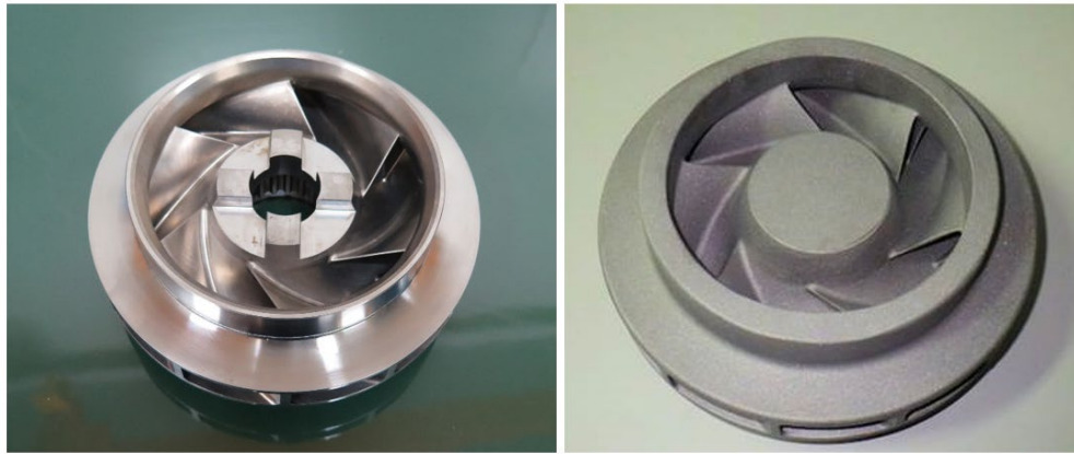
Fig. 4: Machined/brazed impeller (left) and investment casted impeller (right)
