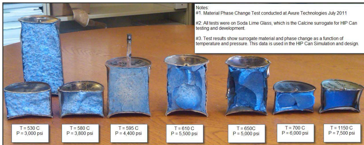
Fig. 9. Vertical cuts of all cans showing various volumetric reductions.
