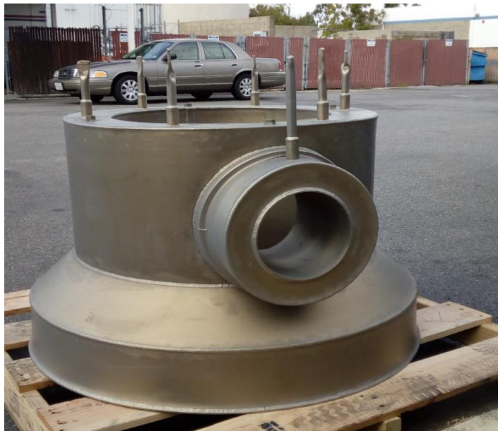
Figure 6. A508 SMR Steam Access Port produced via PM-HIP.
