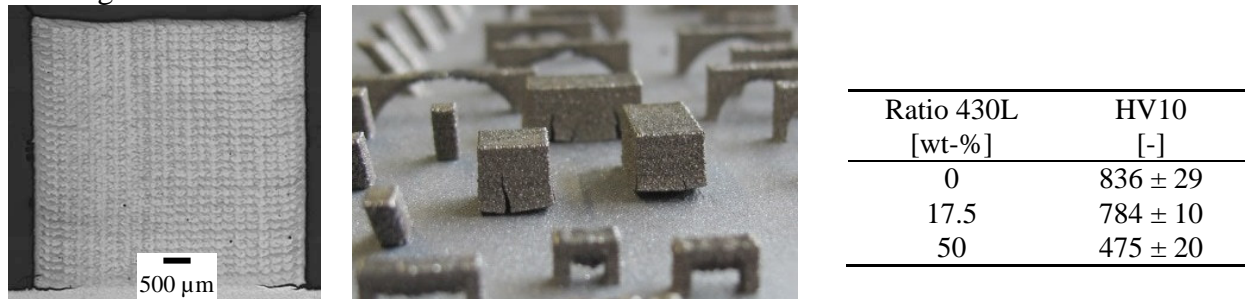
Figure 2: Nearly crack-free cube of A11 + 17.5 wt-% 430L (left); small parts of A11 + 50 wt-% 430L (middle); hardness HV10 of A11 and mixtures (right).
