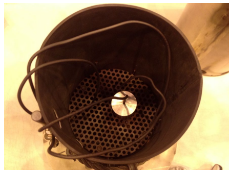
Figure 6. Set up of sample with thermocouple in the HIP furnace.
