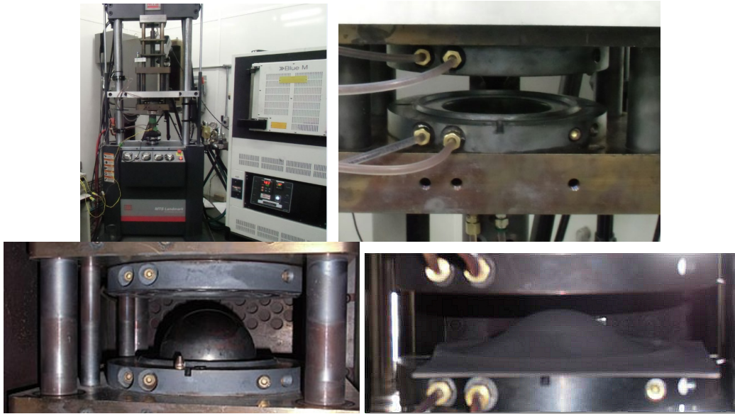
Figure 2: Four-inch Nakazima set-up for hot stamping trials.
