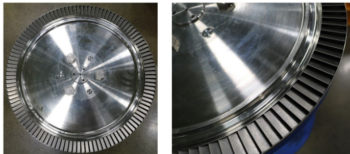
Fig. 3: Blades and shroud made by EDM machining
