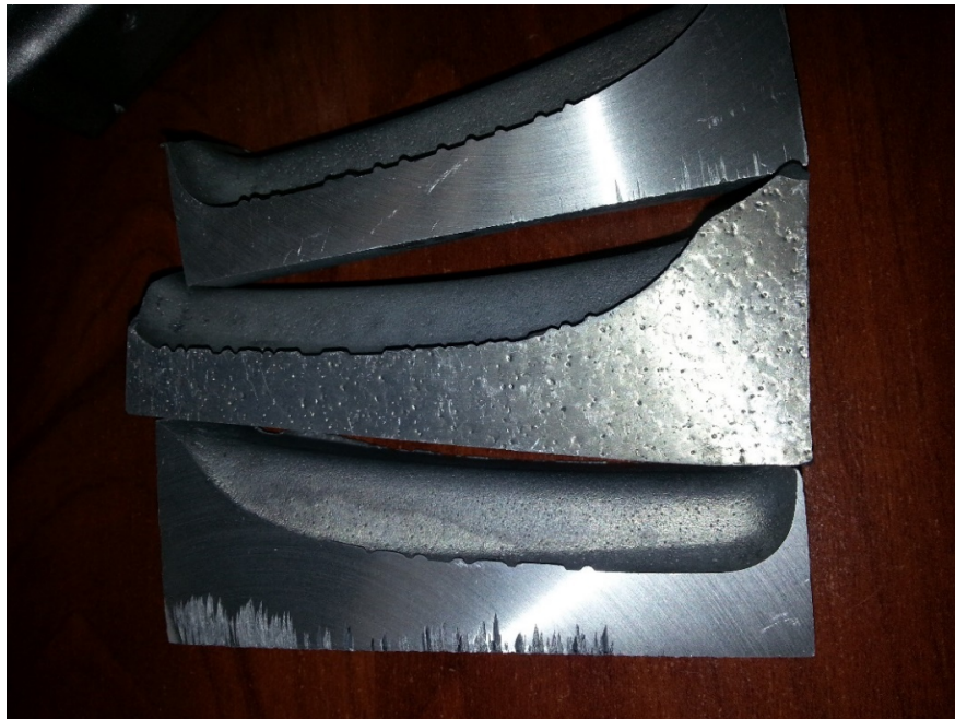
Figure 1. Material before HIP (in the middle) and after HIP (top/bottom).
