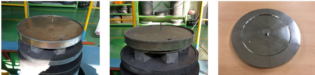
Fig. 2: Canned metal powder before HIP(left), after HIP(center) and machined disk(right)
