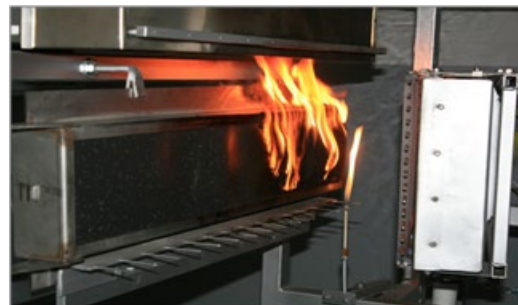
Fig.6. Test according to ISO 5658-2 (determination of CFE) for EPDM.
