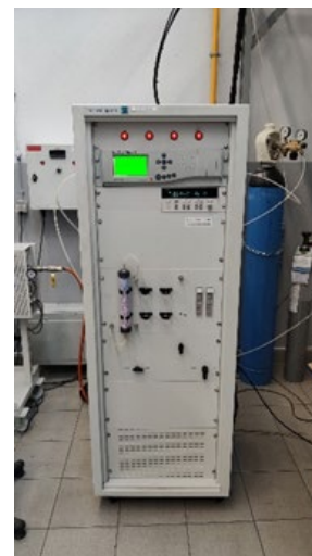
Fig. 2 Rack with oxygen analyzer
