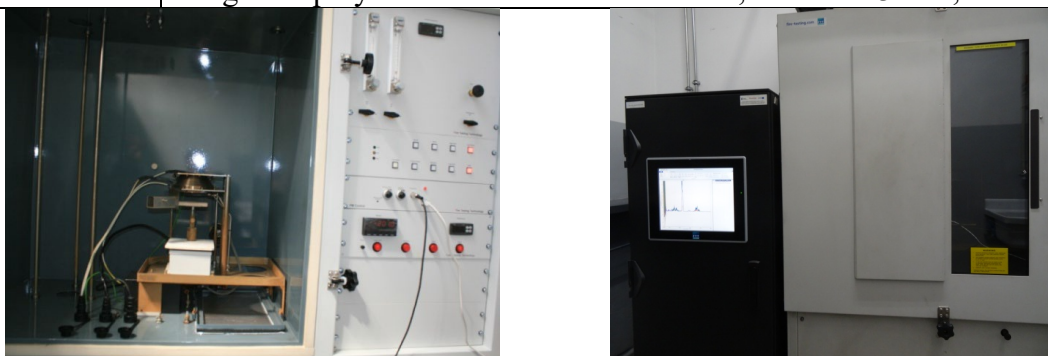
Fig. 1 Smoke chamber (on the left) and FTIR analyzer conjugated with it for determination of gas toxicity according to PN-EN 45545-2:A1:2015 [1] (source: Materials & Structure Laboratory Instytut Kolejnictwa)
