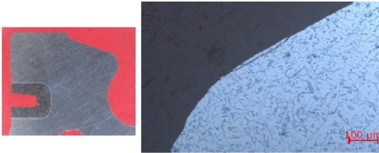
Figure 4. The result of metallographic research - a near-surface material
