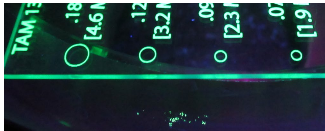
Fig. 1. The cluster of porosity on the turbine nozzle outlet.
